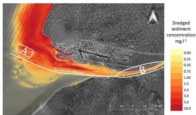
Fig. 1: Percentile 50 over a semi-diurnal tidal cycle of the marked suspended mud concentration ( i.e. previously dredged in the navigation channel ) at the Seine estuary mouth. Dredged sediment marking started 6 months before. Area A represents the dumping site of Rouen harbour. The estuary turbidity maximum zone is located in area B at this period of the year, and extends seawards for high river discharge.
