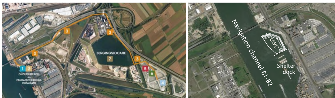
Fig. 1: AMORAS production sites (left): 1. under water cell, 2. Sand separation, 3. Piping, 4. Consolidation ponds, 5. Dewatering installation, 6. Water treatment, 7. Storage. Right: Location of the underwater cell in the shelter dock for push-tow barges
