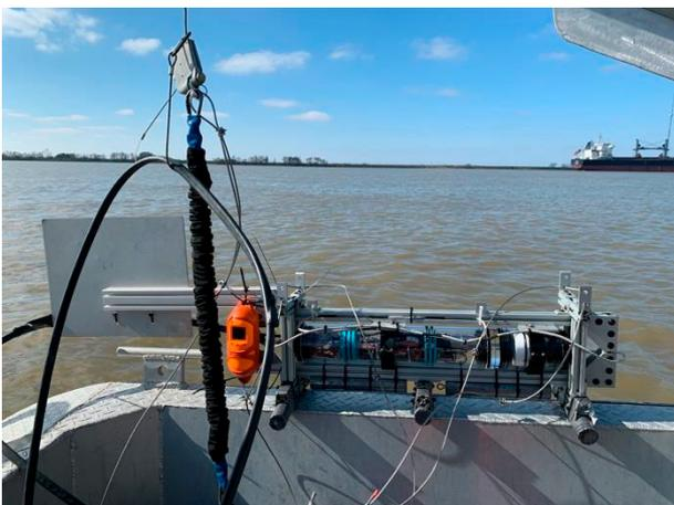
Figure 1: the FLOC AREa and siZing Instrument (FLOCARAZI).
