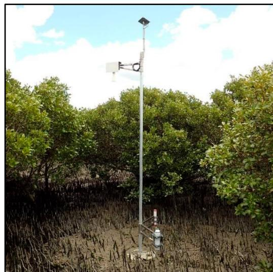
Figure 1: Deployed frame with ASED sensor in the Firth of Thames mangroves. Picture taken in December 2019.
