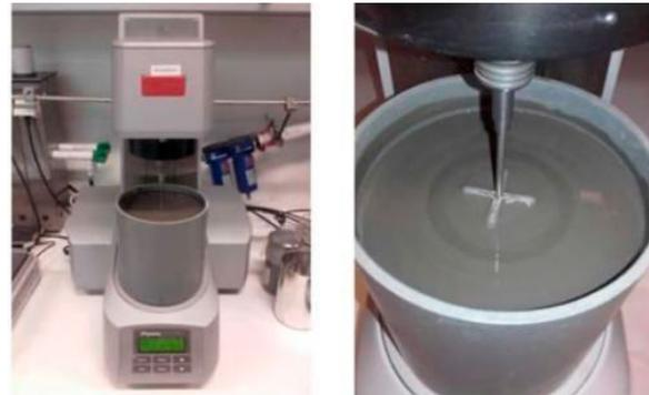
Figure 1: Wide gap vane rheometer setup.
