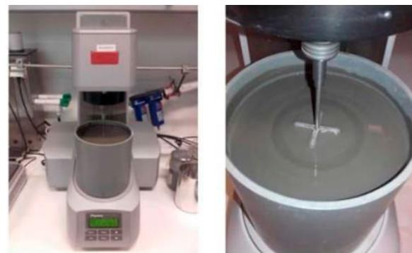
Figure 1: Wide gap vane rheometer setup.
